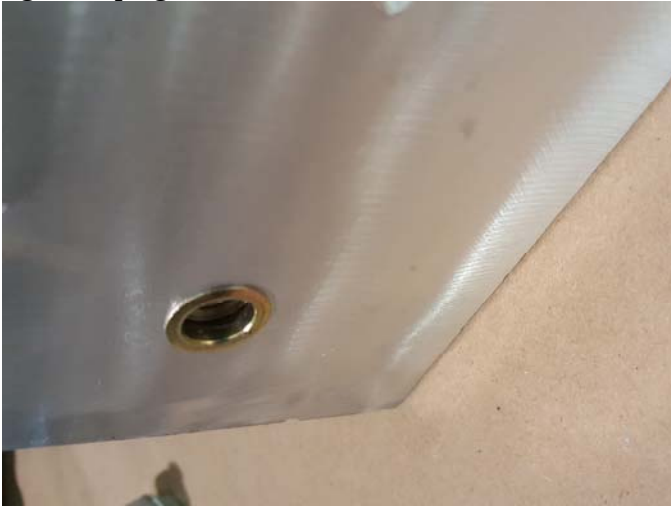
Figure 6: rivet nut correctly installed front side.
