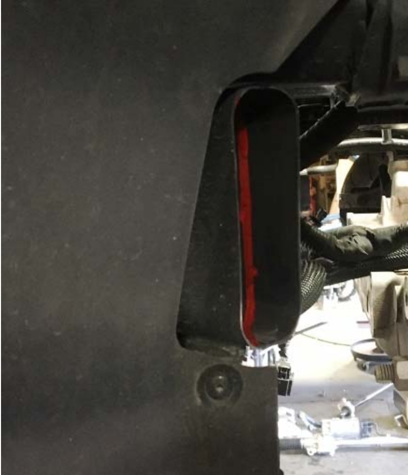
Figure 11: OEM duct marked to be trimmed.
