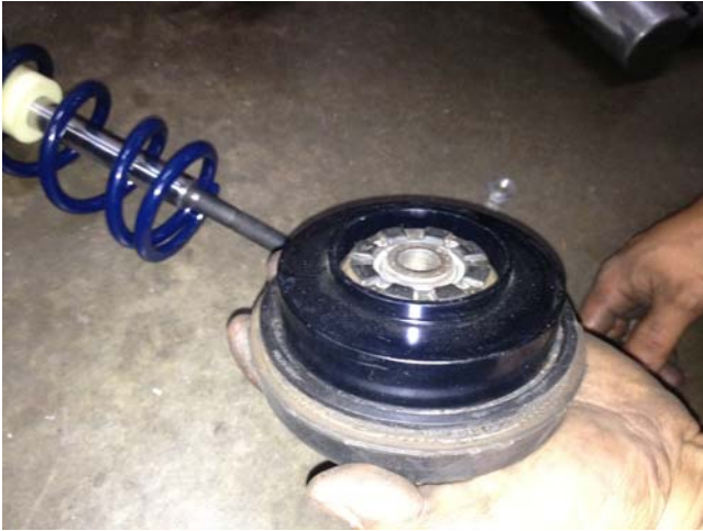
Figure 18: LG spring mount adapter installed on OEM bearing
