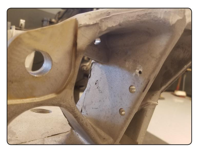
Install tie rod bracket and tighten both bolts to the subframe. Reinstall pin to spindle.
